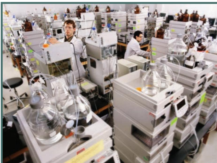
**Figure 1.** PPD cGMP laboratories have more than 230 high-performance liquid chromatography (HPLC) instruments to provide analytical capabilities such as method development, validation, stability and QC testing for clients.
