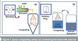
melt extrusion process (used in Zmax<sup>®</sup>) and b) spray congealing with cryogenic solvent extraction (used with Nutropin Depot<sup>®</sup>).
